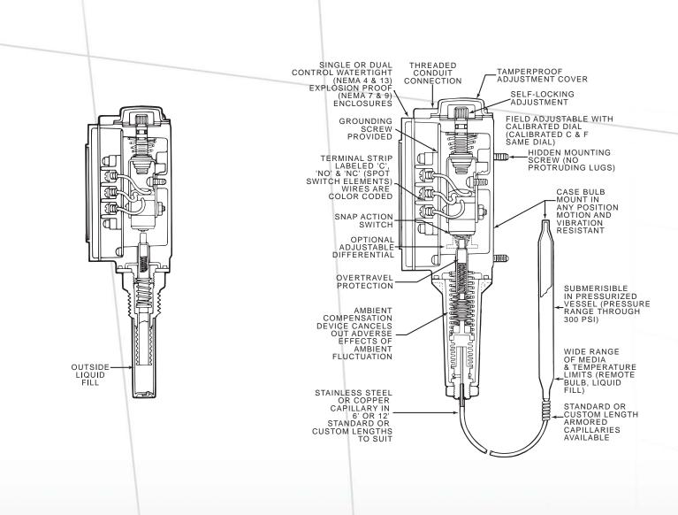
Barksdale offers both remote and local mount temperature switches in housed, NEMA 4 and/or explosion proof designs. All are available with one or two adjustable temperature set points and fixed or adjustable differential.
